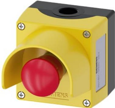
Enclosure for command devices, 22 mm, round, Enclosure material metal, Enclosure top part yellow, with protective collar, 1 control point metal, A=EMERGENCY STOP mushroom pushbutton red, 40 mm, rotate-to-unlatch, 1 NO, 1 NC, 1 NC, screw terminal, floor mounting, 1xM20 each on top and bottom
