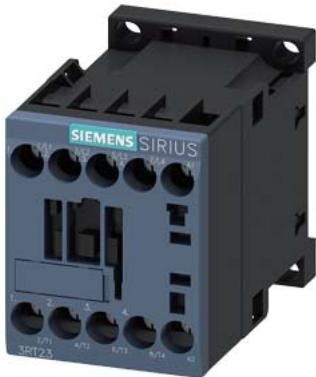
Contactor, AC-1, 18 A/400 V/40 °C, S00, 4-pole, 220 V AC/50 Hz, 240 V/60 Hz, screw terminal
