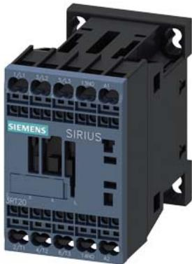
Power contactor, AC-3 7 A, 3 kW / 400 V 1 NO, 220 V AC, 50 Hz 240 V, 60 Hz, 3-pole, Size S00, Spring-type terminal upright mounting position
