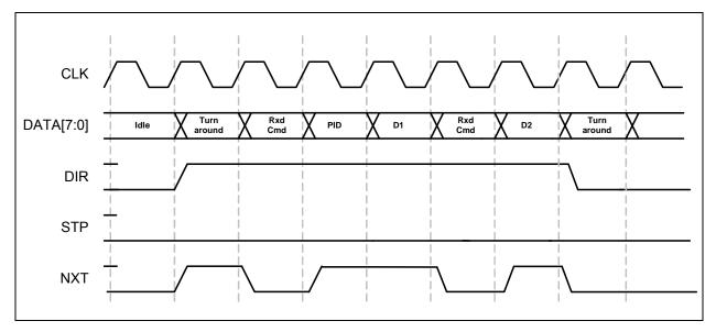
In Figure 6-8 the PHY asserts **DIR** to take control of the data bus from the Link. The assertion of **DIR** and **NXT** in the same cycle contains additional information that Rxactive has been asserted. When **NXT** is de-asserted and **DIR** is asserted, the RXCMD data is transferred to the Link. After the last byte of the USB receive packet is transferred to the PHY, the linestate will return to idle.
