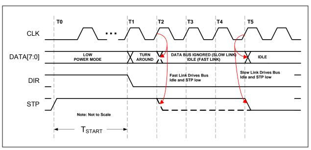
FIGURE 6-12: EXITING LOW POWER MODE
