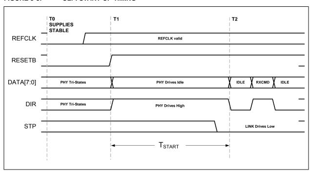
FIGURE 5-8: ULPI START-UP TIMING
