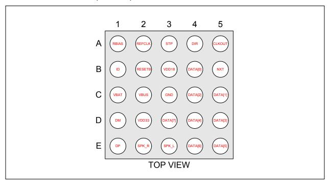
FIGURE 2-2: USB3330 BALL LOCATIONS - TOP VIEW
