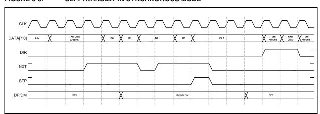
FIGURE 6-9: ULPI TRANSMIT IN SYNCHRONOUS MODE
