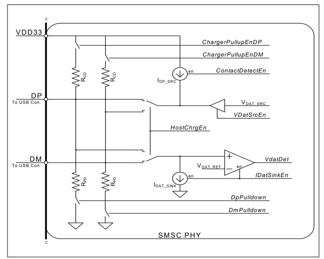
FIGURE 5-11: USB CHARGER DETECTION BLOCK DIAGRAM
