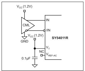
**FIGURE 7-2:** CML Interface (DC-Coupled, 1.2V).
