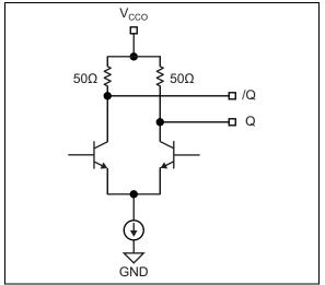
FIGURE 6-4: Simplified CML Output Buffer.
