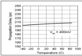
**FIGURE 2-2:** Propagation Delay vs. Temperature.
