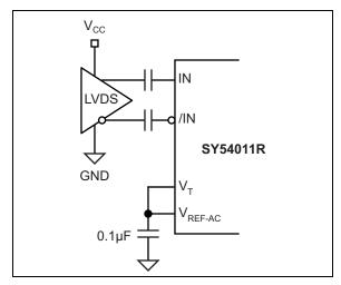
FIGURE 7-7: LVDS Interface (AC-Coupled).
