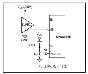
FIGURE 7-5: LVPECL Interface (DC-Coupled).
