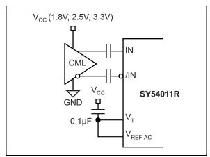
FIGURE 7-3: CML Interface (AC-Coupled).
