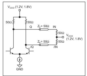
FIGURE 8-1: 1.2V or 1.8V CML DC-Coupled Termination.
