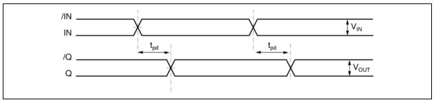
FIGURE 6-1: Propagation Delay.
