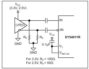
FIGURE 7-4: LVPECL Interface (AC-Coupled).
