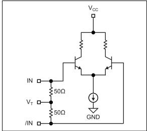
FIGURE 6-2: Simplified Differential Input Buffer.
