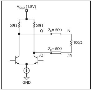
**FIGURE 8-2:** 1.8V CML DC-Coupled Termination.
