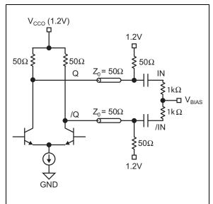
FIGURE 8-4: CML AC-Coupled Termination (V<sub>CCO</sub> 1.2V Only).
