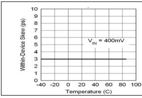
**FIGURE 2-3:** Within-Device Skew vs. Temperature.
