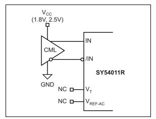
FIGURE 7-1: CML Interface (DC-Coupled, 1.8V, 2.5V).
