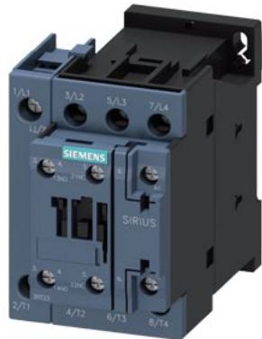
Contactor, AC-1, 50 A/400 V/40 °C, S0, 4-pole, 110 V AC/50 Hz, 120 V/60 Hz, 1 NO+1 NC, screw terminal
