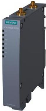
IWLan Access Point, SCALANCE W774-1 RJ45, 1 radio, 2 R-SMA antenna port, iFeatures support via key plug, IEEE 802.11a/b/g/h/n, 2.4/5GHz, gross data rate 300 Mbit/s, 2x RJ45 max. 100 Mbit/s, PoE integrated 2-port switch, redundant 24 V DC, terminal block, IP30, -20... 60 °C, plug slot WPA2/802.11i/e, observe national approvals! CERT ID: MSN-W1-RJ-E2, scope of delivery: Manuals on CD-ROM, German/English, 1x terminal block; for operation in the USA
