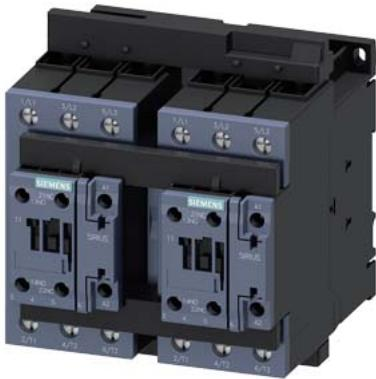
Reversing contactor assembly AC-3, 37 kW/400 V 110 V AC 50 Hz/120 V 60 Hz, 3-pole Size S2, screw terminal electrical and mechanical Interlock 2 NO integrated
