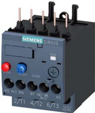
Overload relay 0.14...0.20 A Thermal For motor protection Size S00, Class 10 Contactor mounting Main circuit: Screw Auxiliary circuit: Screw Manual-Automatic-Reset
