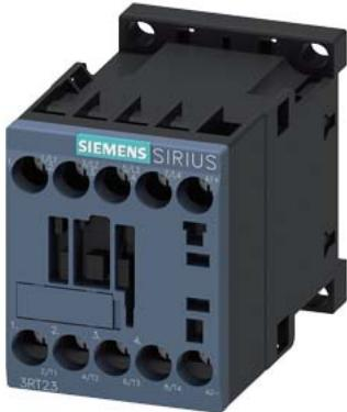
Contactor, AC-1, 22 A/400 V/40 °C, S00, 4-pole, 24 V DC, screw terminal
