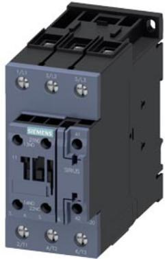
Power contactor, AC-3 80 A, 37 kW / 400 V 1 NO + 1 NC, 24 V DC with varistor 3-pole, Size S2 Screw terminal Suitable for 2 A PLC outputs
