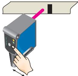
When setting the contrasts to be detected, the second LED (green) flashes in the bar graph.
