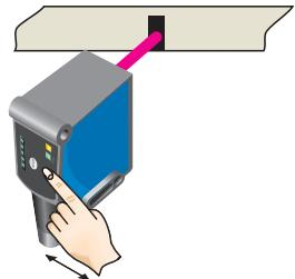
When setting the contrasts to be detected, the first LED (green) flashes in the bar graph.
