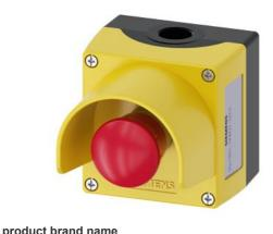
Enclosure for command devices, 22 mm, round, Enclosure material metal, Enclosure top part yellow, with protective collar, 1 control point metal, A=EMERGENCY STOP mushroom pushbutton red, 40 mm, rotate-to-unlatch, 1 NC, 1 NC, screw terminal, floor mounting, 1xM20 each on top and bottom
