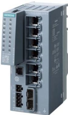
SCALANCE XC206-2SFP G managed Layer 2 IE switch; IEC 62443-4-2 certified; 6x 10/100/1000 Mbps RJ45 ports; 2x 1000 Mbps SFP; 1x console port; diagnostics LED; redundant power supply; temp. range -40 °C to +70 °C; mounting: DIN rail/S7 mounting rail/wall; redundancy functions; Office features (RSTP, VLAN,...); PROFINET IO device; Ethernet/IP-compliant; C-plug slot;
