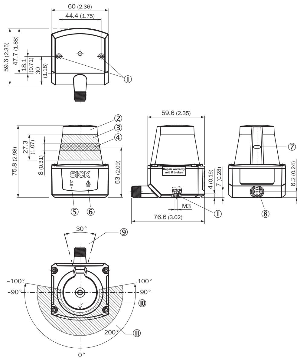
① M3 threaded mounting hole, 2.8 mm deep (blind hole thread), max. tightening torque 0.7 Nm
