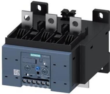
Overload relay 50...200 A for motor protection Size S6, CLASS 5...30E
