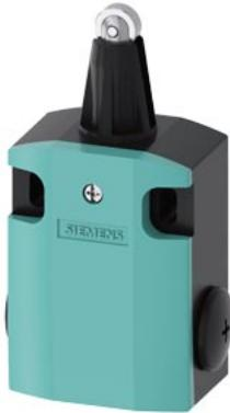
Position switch Metal enclosure 56 mm wide, Device connection 3x (M20x 1.5) 1 NO/1 NC quick action contacts, Roller plunger with 3 mm overtravel, Stainless steel roller 13 mm
