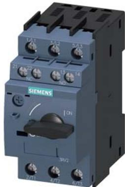
Circuit breaker size S00 for motor protection, CLASS 10 A-release 1.8...2.5 A N-release 33 A screw terminal Standard switching capacity with transverse auxiliary switches 1 NO+1 NC
