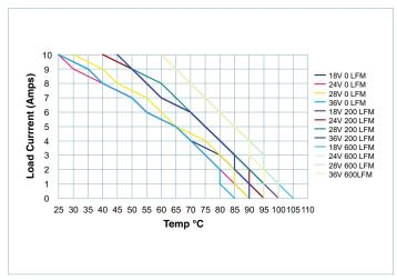
Figure 2 — Load currrent vs. temperature (without heat sink)
