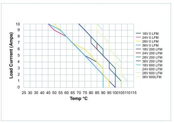
**Figure 4** — Load currrent vs. ambient temperature (11mm heat sink)
