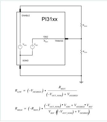
Figure 22 — Trim equations and equivalent circuit
