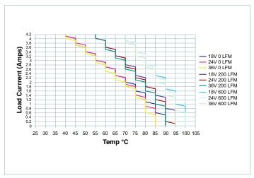
Figure 12 — Load currrent vs. temperature (without heat sink)
