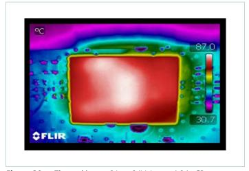
**Figure 20** — Thermal image ( $V_{IN} = 24V$ ,  $I_{OUT} = 4.2A$ , CR, OLFM evaluation PCB)
