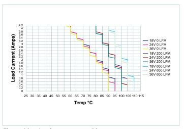
**Figure 14** — Load currrent vs. ambient temperature (11mm heat sink)
