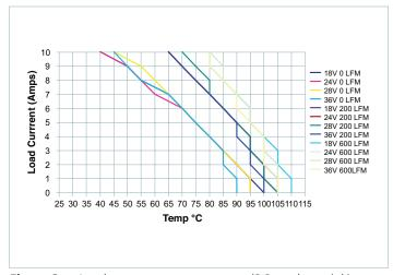
Figure 3 — Load currrent vs. temperature (6.3mm heat sink)
