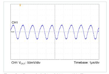
**Figure 9** — Output ripple ( $V_{IN} = 24V$ ,  $I_{OUT} = 10A$ , CR,  $C_{OUT} = 6 \times 10 \mu F X7R$  ceramic)
