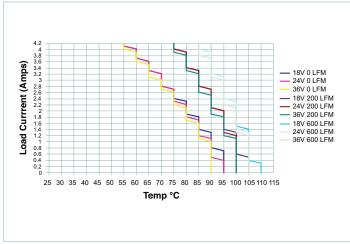
Figure 13 — Load currrent vs. temperature (6.3mm heat sink)
