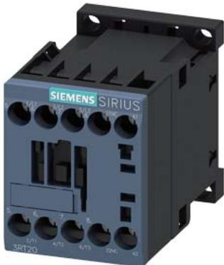
Power contactor, AC-3 9 A, 4 kW / 400 V 1 NC, 24 V AC, 50 / 60 Hz 3-pole, Size S00 screw terminal
