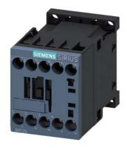
Contactor, 2NO + 2NC, AC-3, 4 kW 110 V AC, 50 Hz, 120 V, 60Hz, 4-pole, 2NO + 2NC, Size S00, Screw terminal
