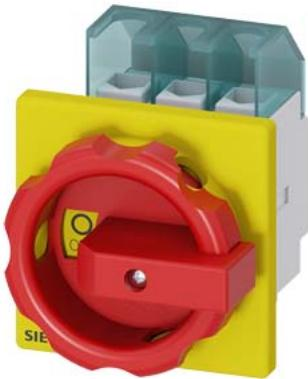
SENTRON, Switch disconnector 3LD, emergency switching-off switch, 3-pole, I<sub>u</sub>: 25 A, operating power / at AC-23 A 400 V: 9.5 kW, front-mounted, rotary operating mechanism, Red / yellow, 4-hole mounting of the handle
