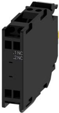
Contact module with 1 contact element, 1 NC, Contact for installation monitoring, spring-type terminal, for front plate mounting
