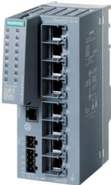
SCALANCE XC208 managed Layer 2 IE switch; IEC 62443-4-2 certified; 8x 10/100 Mbps RJ45 ports; 1x console port; diagnostics LED; redundant power supply; temp. range -40 °C to +70 °C; mounting: DIN rail/S7 mounting rail/wall Office redundancy functions features (RSTP, VLAN,...); PROFINET IO device Ethernet/IP-compliant C-plug slot;
