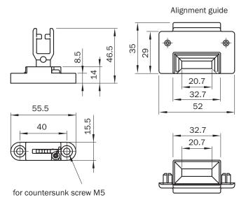
Semiflexible method of actuation: The actuator facilitates movement in the horizontal plane only.
