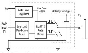
Figure 1: Block Diagram of EPC9002 Development Board
