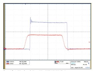
Figure 4: Typical Waveforms for V $_{\rm IN}=48\,{\rm V}$  to 5 V/7 A (500kHz) Buck converter CH1: Switch node voltage (Vsw) - CH2: PWM input voltage (V $_{\rm PWM}$ )
