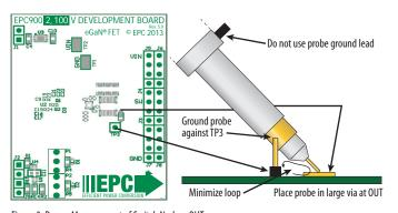
Figure 3: Proper Measurement of Switch Node — OUT
