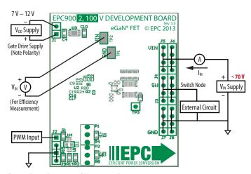
Figure 2: Proper Connection and Measurement Setup
