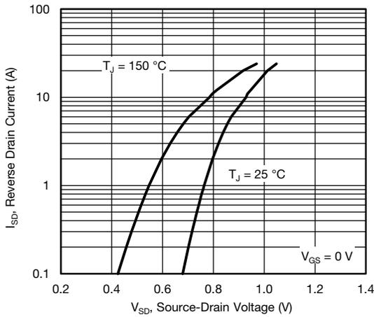
**Fig. 8 - Typical Source-Drain Diode Forward Voltage**
