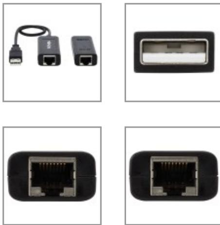
Connects your home/office PC or laptop to a webcam, printer, hard drive or other USB 2.0 peripheral located up to 164 ft. away.
