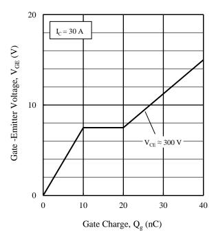
Figure 12. Typical Gate Charge
