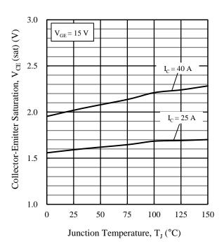
Figure 9. Saturation Voltage vs. Junction Temperature
