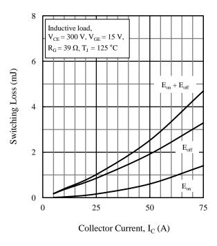
Figure 17. Switching Loss vs. Collector Current
