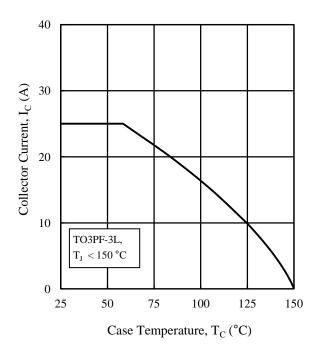
Figure 5. Collector Current vs. Case Temperature
