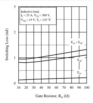
Figure 18. Switching Loss vs. Gate Resistor
