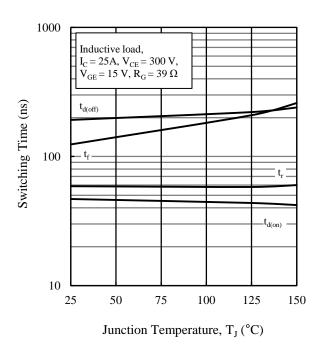
Figure 13. Switching Time vs. Junction Temperature
