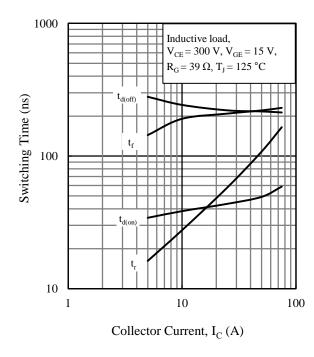
Figure 14. Switching Time vs. Collector Current
