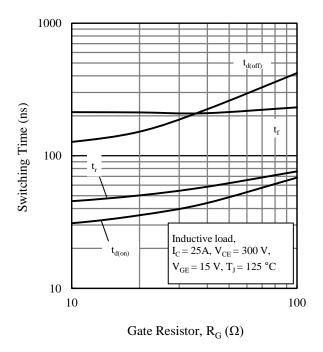
Figure 15. Switching Time vs. Gate Resistor
