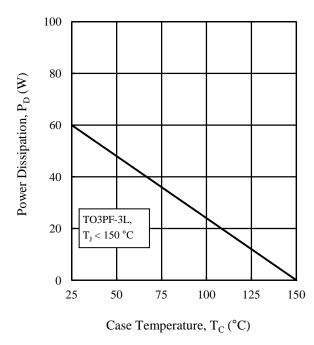
Figure 4. Power Dissipation vs. Case Temperature
