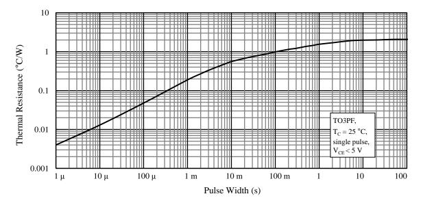
Figure 19. Transient Thermal Resistance
