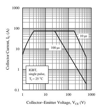
Figure 3. IGBT Safe Operating Area
