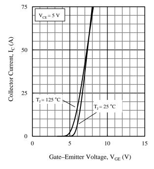
Figure 8. Transfer Characteristics
