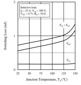
Figure 16. Switching Loss vs. Junction Temperature
