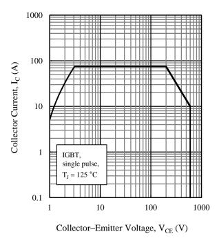
Figure 2. IGBT Reverse Bias Safe Operating
