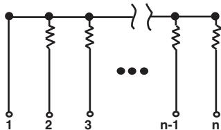
5, 7 or 9 resistors with one pin common
