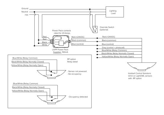
1 Circuit with up to 4 Sensors and UVPP
