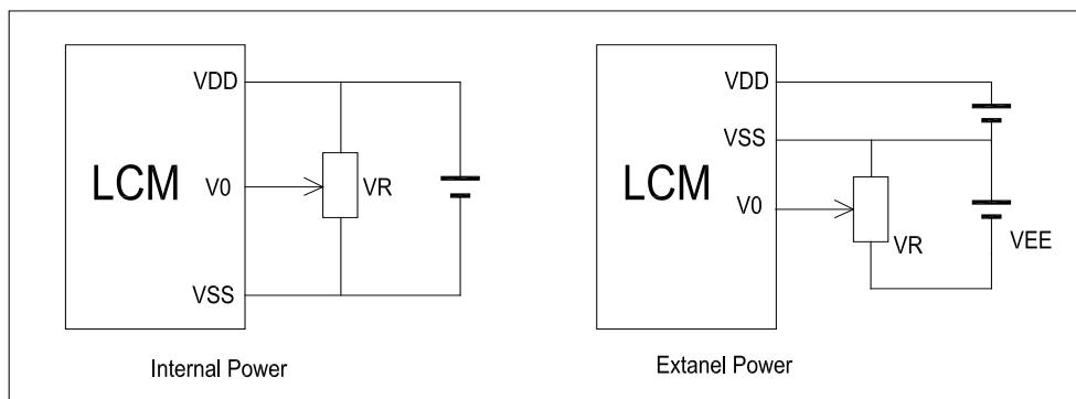
$V_{DD}-V_0$ : LCD Driving voltage
