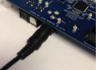
Figure 11. Connecting the Power Supply
