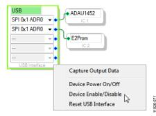
Figure 69. Toggling the Reset Signal in SigmaStudio
