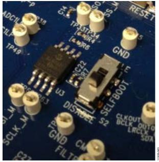
Figure 61. Self-Boot EEPROM and Slide Switch
