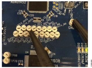
Figure 58. Monitoring Digital Audio Signals from the Test Points
