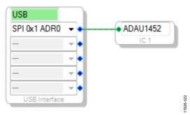
Figure 20. Connecting the USBi to an ADAU1452 in the Hardware Configuration Tab
