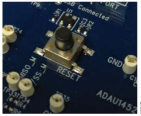
Figure 68. Manual Reset Push-Button and Reset Generator IC
