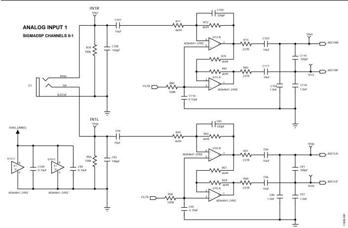
Figure 79. Analog Input Channel 0 and Channel 1
