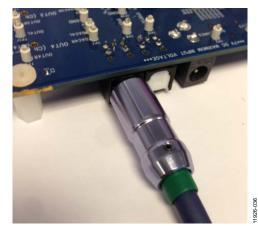
Figure 34. Photograph of the Optical S/PDIF Input Connection
