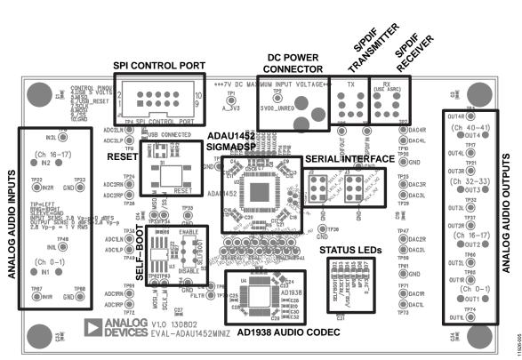
Figure 3. Board Layout Block Diagram
