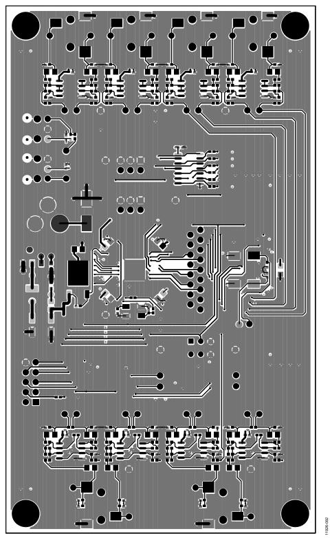
Figure 90. EVAL-ADAU1452MINIZ Layout, Bottom Copper
