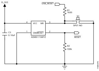
Figure 77. Reset Generator Circuit
