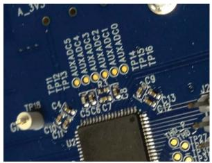
Figure 60. Copper Pads for Inputting Signals to the Auxiliary ADC
