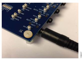
Figure 14. Analog Stereo Output Connection
