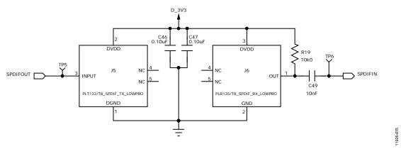
Figure 73. S/PDIF Optical Interfaces
