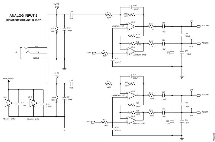
Figure 80. Analog Input Channel 16 and Channel 17
