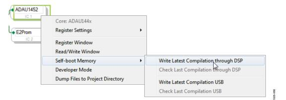
Figure 64. Writing to the EEPROM Through the ADAU1452 Master SPI Port
