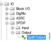
Figure 48. S/PDIF Output Block Selection
