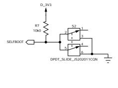
Figure 72. Self-Boot Circuit
