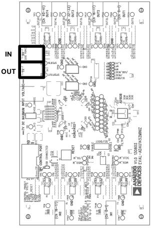
Figure 33. Location of S/PDIF Optical Input (J5) and Output (J6), Rotated 90°
