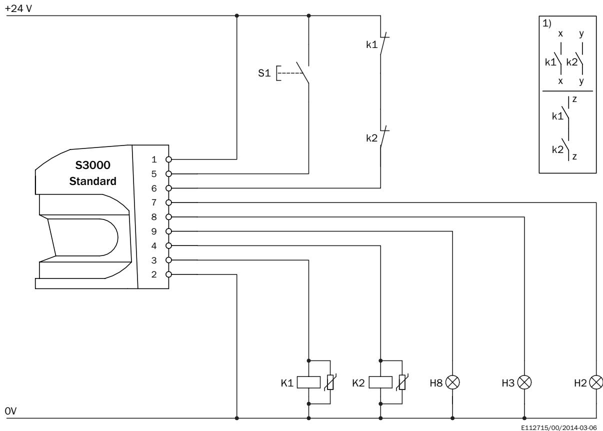
S3000 Standard in conjunction with relays/contactors
