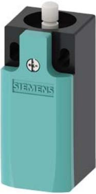
position switch plastic enclosure according to EN 50047, 31 mm device connection 1 x (M20 x 1.5) 1 NO/1 NC quick-action contacts integrated (not replaceable) rounded plunger form B with rounded plunger
