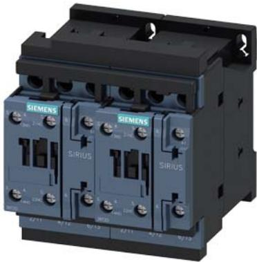
Reversing contactor assembly AC-3, 11 kW/400 V 110 V AC 50 Hz/120 V 60 Hz, 3-pole Size S0, screw terminal electrical and mechanical Interlock 2 NO integrated
