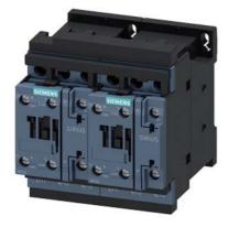
Reversing contactor assembly AC-3, 7.5 kW/400 V 110 V AC 50 Hz/120 V 60 Hz, 3-pole Size S0, screw terminal electrical and mechanical Interlock 2 NO integrated
