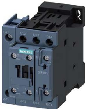
Contactor, AC-1, 35 A/400 V/40 °C, S0, 4-pole, 24 V DC, 1 NO+1 NC, screw terminal
