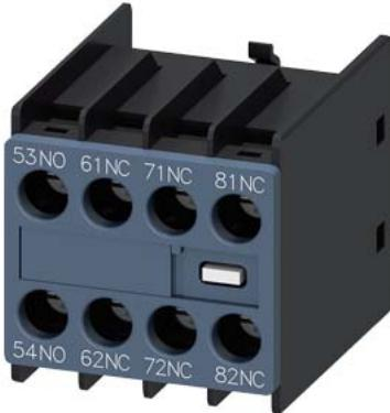
Auxiliary switch on the front, 1 NO + 3 NC Current path 1 NO, 1 NC, 1 NC, 1 NC for contactor relays Size S00 screw terminal 51/52, 61/62, 71/72, 81/82 Physically coded; only with contactor relays 3RH2140\* and 3RH2440\* can be combined (according to EN 50011)
