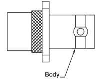
3) Solder the contact onto the centre conductor.
