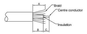
2) Slide the hex nut, washer and grommet over the cable. Place the taper clamp over the braid and push back against the cable jacket. Pull the braid back over the taper clamp and trim level with the rear as shown.
