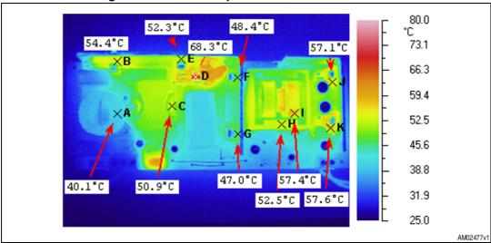
Figure 16. Thermal map at 115 Vac - 60 Hz - full load
