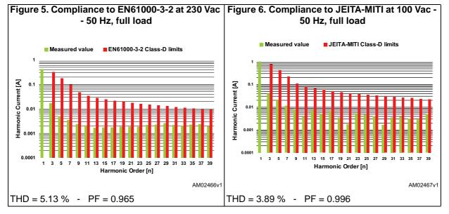
On the bottom side of the diagrams the total harmonic distortion and power factor have also been measured. The values in all conditions give a clear idea about the correct functioning of the PFC.
