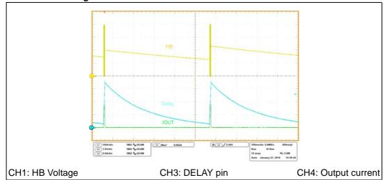
Figure 15. Short-circuit at full load and 115 Vac - 60 Hz
