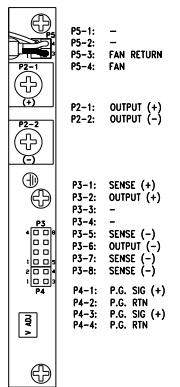
**P2:** 10-32 screw down terminal mates with #10 ring tongue terminal. (10 in-lb Max)
