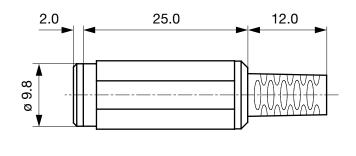
Cable diameter max. 4.0 mm
