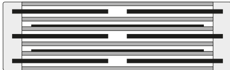
Extended foil design with internal series connection and metallized film (series connection of 2 elements)
