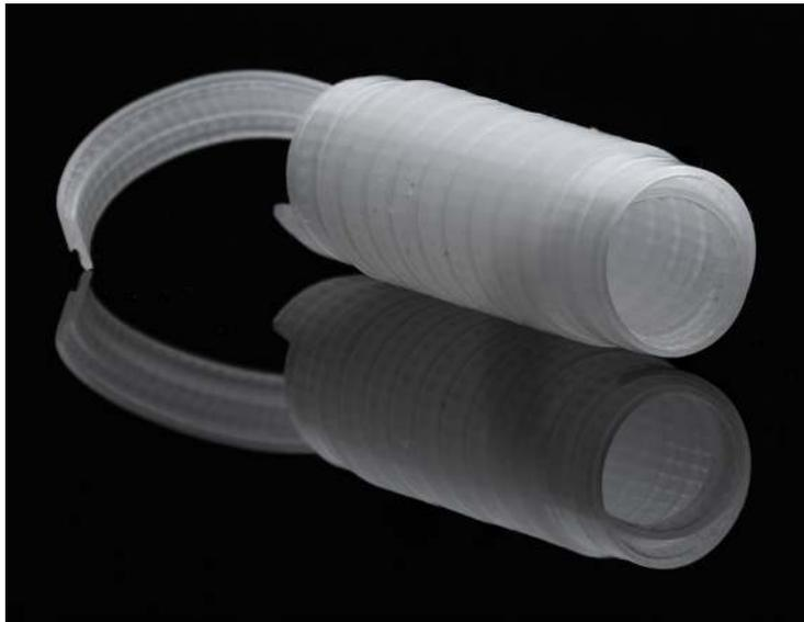
Gamma's Clear SDL Cold Shrink Tubing is a specially formulated, pre-expanded transparent silicone rubber shrink tubing that does not require heat to shrink. It is intended for weatherproofing of AC & DC electrical power wire/lug assemblies. This transparent silicone rubber allows the integrity of the waterproof seal on the wire/lug interface to be
