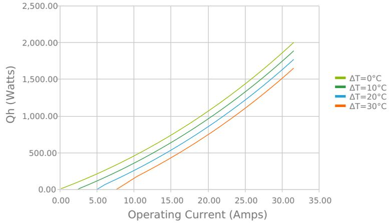
Total Heat Dissipated at Hot Side (Qh=Qc+Pin)
