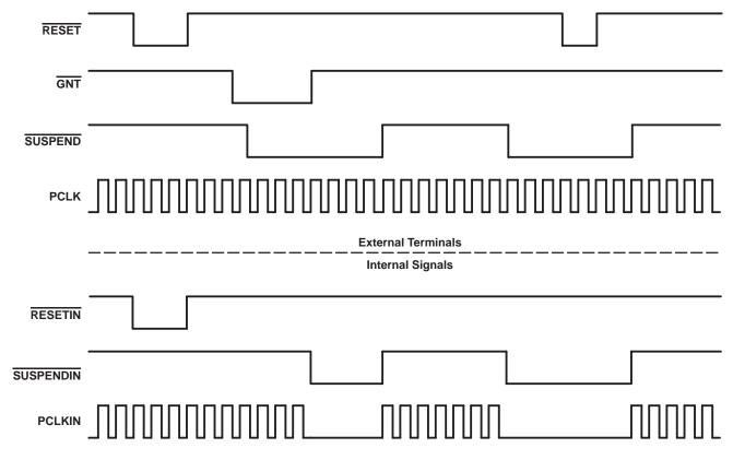
Figure 3-13. Signal Diagram of Suspend Function
