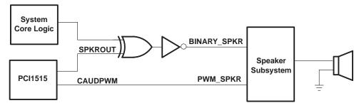
Figure 3-4. SPKROUT Connection to Speaker Driver
