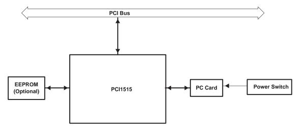
Figure 3-1. PCI1515 System Block Diagram
