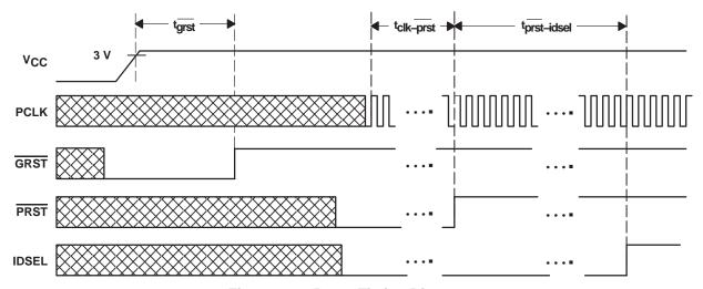
Figure 7–1. Reset Timing Diagram
