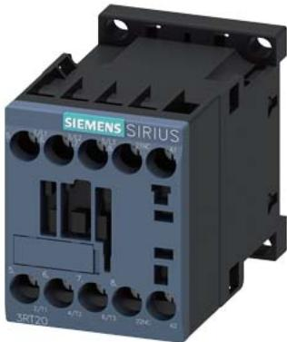
Power contactor, AC-3 12 A, 5.5 kW / 400 V 1 NC, 110 V AC, 50 Hz, 120 V 60 Hz, 3-pole, Size S00 screw terminal
