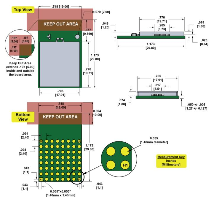
Fig. 1: SM200PF1/PU1 Mechanical Drawing
