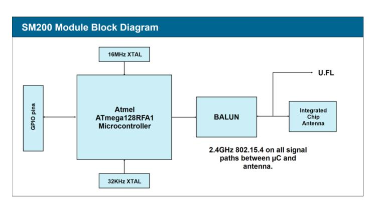
Fig. 2: Block diagram showing the major subsystems comprising Model SM200
