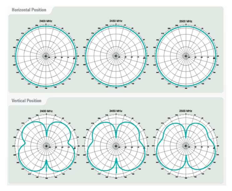
Fig. 2: Pulse W1027 Antenna Gain Performance
