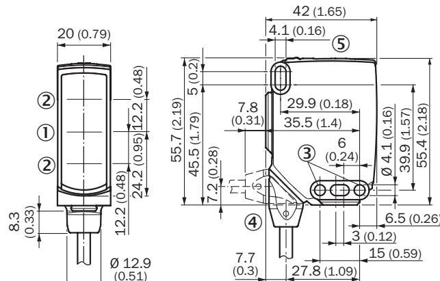
① Center of optical axis, sender
